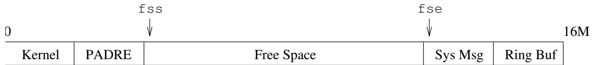
Figure 1: Top Level Allocation Of Cell Memory. Kernel represents the space used by the cell operating system, PADRE represents the space needed for the PADRE cell program and its stack, and Sys Msg and Ring Buf the space needed for message-passing buffers. Note that Ring Buf is not used by PADRE and may be of zero length.
